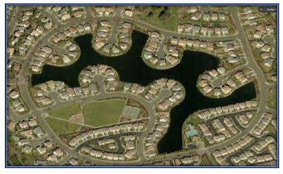
of the lake that is connected to the City storm drain system. Water leaving the lake travels through a series of storm drain pipes which eventually drain into Green Valley Creek. Water from Green Valley Creek drains into Cordelia Slough which eventually drains into Suisun Slough which then drains into Suisun Bay.
