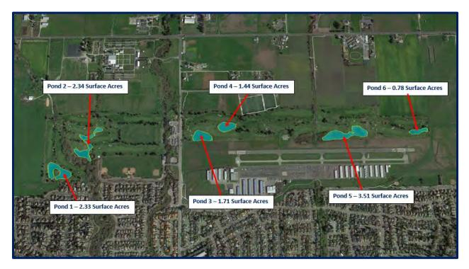
The ponds are primarily filled by a well and also are fed by rainfall and storm runoff from the surrounding storm water system. The ponds are maintained as a static system during the summer months by maintaining them below the spillway. All six (6) of the ponds are connected to each other through a pipe system so they are all connected and flow from one to another. Pond #2 is the last pond in the chain of connected ponds and has a spillway that is connected to Lynch
