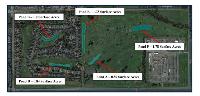
The ponds are primarily filled by rainfall in the winter, in the summer they are filled with reclaimed water from Ellis Creek. Ponds D and F are used for irrigation, while ponds A and B are ornamental. Pond A does not discharge and Pond B discharges directly into the city's wastewater system. Ponds D, E, and F are chained such that Pond F discharges into Pond E, Pond E discharges into Pond D, and Pond D discharges into the city's wastewater system.
