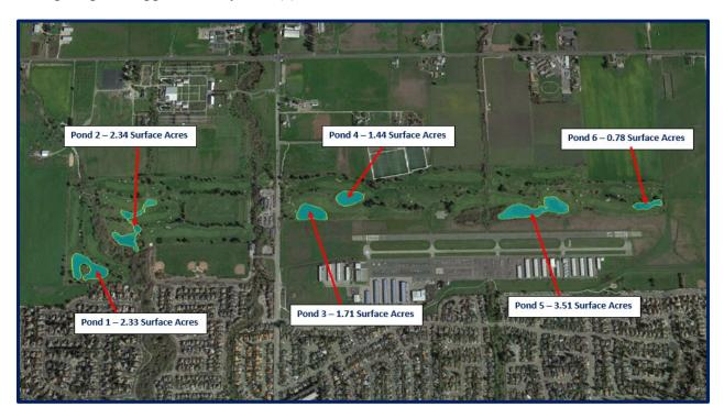
The ponds are primarily filled by a well and are fed by rainfall and storm runoff from the surrounding storm water system. The ponds are maintained as a static system during the summer months by maintaining them below the spillway. All six (6) of the ponds are connected to each other through a pipe system so they are all connected and flow from one to another. Pond #2 is
