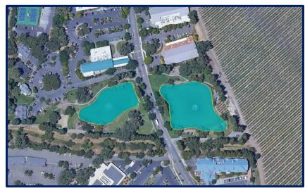
in the winter for storm events. Water leaves the ponds primarily from irrigation but when the pipes are uncapped for storm events the water drains into an unnamed creek which then flows into Windsor Creek which flows into Mark West Creek which eventually flows into the Russian River.
