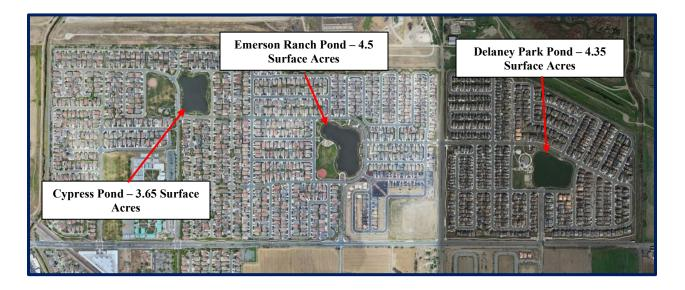
During the summer, water for the pond will be supplied from groundwater. During the wet season, excess water will exit the pond via pump stations at the edges of each pond and will be discharged into the city's stormwater system.
